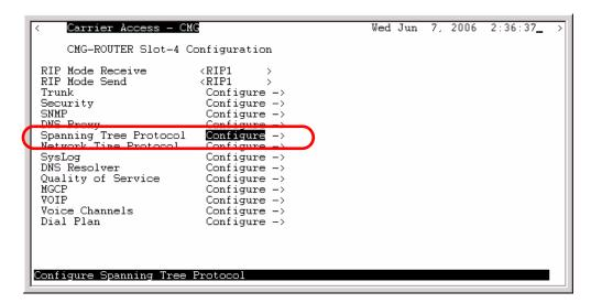
2. To enable Spanning Tree, scroll **<Disabled>** to **<Enabled>**, with the **[SPACEBAR]**, select **[ENTER]**.
